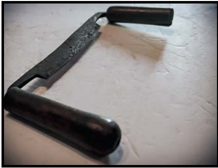
Mast Drawknife (W211-19SCD): One of several examples of this forged, two-handled, bevelled, barrelmaking tool. Used for finishing rough-hewn boards. 1700s.
