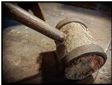
Closer View of Carpenter Beetle (C96-19N): Sturdy wooden mallet with iron banding for reinforcement.
