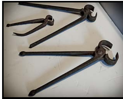
Farrier Nippers (3)(F199-19NEC): Forged iron blacksmith's tools for shoeing horses (and oxen?). Three nippers (also called pincers) are shown in this photograph (2 large and 1 small). Depending on size, these removed nails or old shoe from horse hooves. Mid-1800s.
