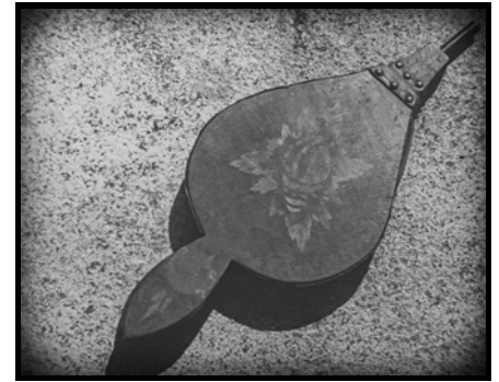
Fireplace Bellows (L132-19SW): For fanning coals into flame: These household bellows are made of wood and leather.
