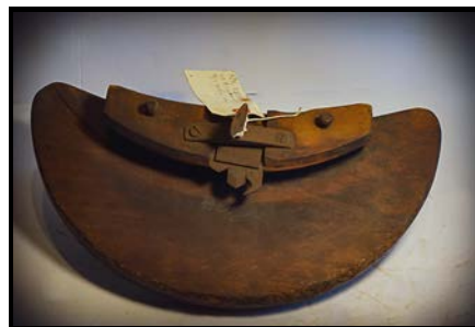
V Groove Croze Plane (C80e-19SW): This croze plane is used to cut a v-groove in wood. 1800s.
