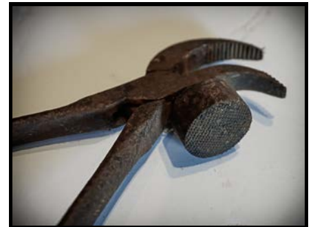
Lasting Pincer (P316-19NEC): Shoemaker's pincer tool with dual purpose: It pulls leather upper over sole and pounds in tacks to hold uppers and soles in place. Early 1800s.
