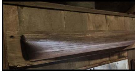
Mounted Half Hull Boat Model (M144-19S): Mounted on display boards, half hull boat models enabled shipwrights to finalize ship designs before initiating construction. 1800s.
