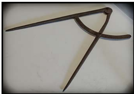
Cooper Divider (T3-19WH): Made of forged iron, this cooper's divider/ compass scribe would have been useful for measuring circles for the base and cover of barrels. 1700s.
