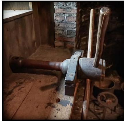
Alternate View of Windlass: Coopers would use a windlass to tighten rope around the top of the barrel staves, holding them in place for hooping (C137-19SW).
