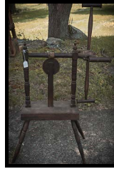
Clock-Style Yarn Skeiner (P32-19SW): Four-legged yarn skeiner with decorative dowels and four arms. In the center of the stand is a saw-toothed circular gear lining up with a horizontal rod ending in a hub into which the skeiner arms are set. The saw teeth in the circle line up with the spiral cuts in the rod, turning the gear to keep track of the wheel's revolutions. 1800s.
