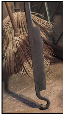
Alternative View of Stock Knife (P62-19NEC): The curved end would be hooked into a block for leverage.
