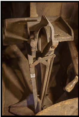
Forged Iron Harness Vice (F101-19NA): Like the wooden harness vice shown earlier, this iron model would have been used to secure sadlery objects for repair. Late 1800s.
