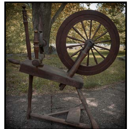
Flax Spinning Wheel (P130-19SW): The distaff (the taller doweled piece at the back), though missing parts, distinguishes this as a flax linen spinning wheel. Early 1800s.
