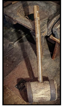
Carpenter Beetle (C96-19N): Striking head is iron-banded on both ends. Useful mallet for carpentry projects. 1800s.
