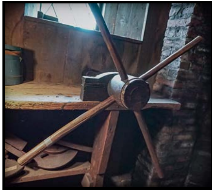
Windlass (C137-19SW): Four-armed wooden windlass used for cinching or hauling. 1700s.
