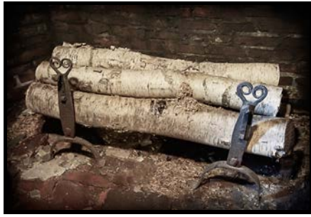
Forged Iron Andirons (L200-19WH): These andirons would have been forged by a blacksmith, perhaps as a bespoke (commissioned) job. The decorative curves and curls on the front surfaces might have served a practical purpose, as well.
