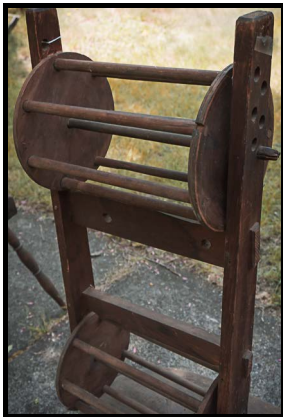
Yarn Reels (P130-19S): This wooden stand with two horizontal doweled reels would have held spun yarn for storage or drying (after dyeing). 1800s.
