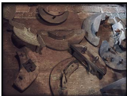
Assorted Barrel Planes (C80-19SW): Depicted here are various styles and periods of barrel planes, including Block, Chamfer, Sun, and Smoothing Planes. 1800s.
