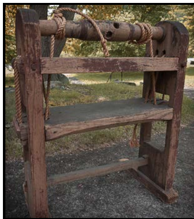
Farm Cheese Press (M113-19SWC): Wooden farm cheese press with rope-driven pulley system. Late 1800s.
