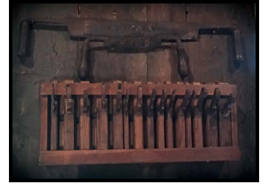
Mast Drawknife (2) (W211-19SCD) and Molding Planes Set (15) (W87-19SCD): These two-handled large and small mast drawknives were used as barrel-planing tools, flattened versions of the open scorper. The 15 molding planes are displayed in an easy-access wooden case. These planes were used to create decorative moldings.
