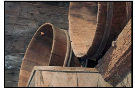
Barrel Tubs of Various Periods (C109-19NER): These barrel tubs can be distinguished primarily by the material used for the binding hoops--either saplings or metal.
