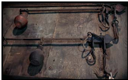
Steelyard Scales (F69-19NW) (F94-19NW): Two sets of balance scales with hooks, balance arms, and counterweights. Used for weighing heavy items. Mid 1800s.
