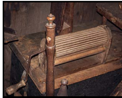
Wooden Clothes Wringer (P90-19NEC): This portable clothing wringer would be set on top of a tub and an item of clothing would be fed through as the handle was turned, squeezing out both water and suds. Late 19th century in construction.
