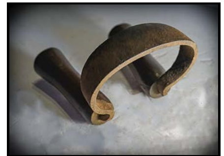
Open Scorper (W22-19SW): Two-handled curved drawknife used in barrelmaking for hollowing out wood and smoothing surfaces. 1800s.
