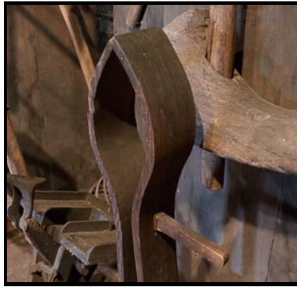
Alternative View of Wood Harness Vice (F88-19NE): Another view of the wooden sadlery harness vice.
