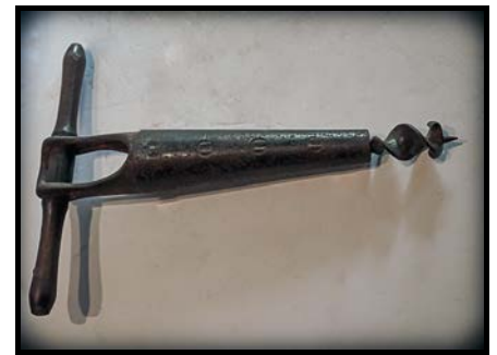
Wheelwright Combination Tool (C16-19CTN): A cast and wrought tool which combines a spiral auger and a reamer. Enables boring and widening a wheel hub at the same time. Originally painted bright red, with a maple wood bar handle. Late 1800s.
