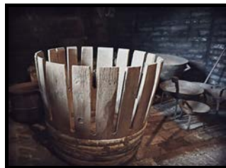
Replica Barrel (C100-19WH) and Three-Legged Iron Skillets (4) (H48128129133-19WH): The unfinished barrel serves as a demonstration of barrel-making. In reality, the staves would have been made from separate pieces, not carved from a single piece as depicted here. Four cast iron skillets, with legs, are visible in the background (late 1700s).
