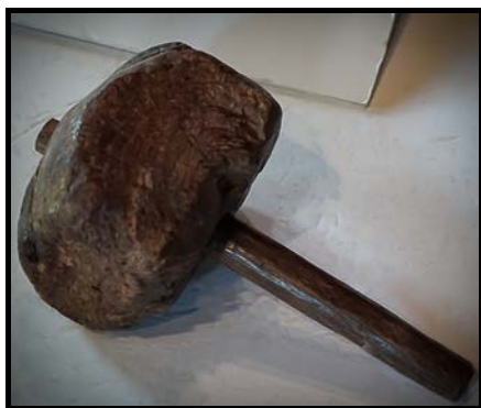
Wheelwright Mallet (C12-19SW): Hammering tool made from a beech burl with a hickory handle. Late 1700s.
