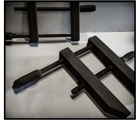
Wood Screw Clamps (2) (W310-19NW): Wood screw clamps such as these adjustable tools were used for woodworking projects. Late 1800s.
