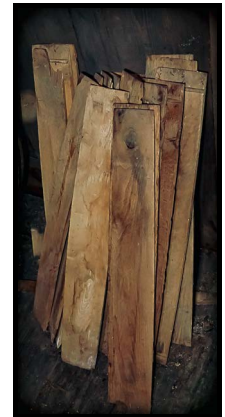
Barrel Staves (W195-19NWC): Barrel staves were often split (rived) from oak by local farmers during the winter, for bartering with the local cooper.
