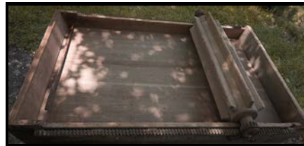
The Philadelphia Butter Worker (P203-19CSW): This butter-making tray, a large rectangular wood pan with high sloping sides and a ribbed roller, has a patent design date of March 13, 1875 and was advertised in the 1893 catalog of the Ames Plow Company.
