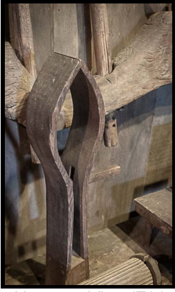
Sadlery Harness Vice (F88-19NE): This wooden harness vice was used to secure a saddle or harness for repairing (especially stitching). Early 1800s.
