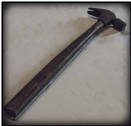
Wrought Iron Claw Hammer (F317-19CTN): Short claw and large head; used for iron nails. Long wood handle. 1800s.
