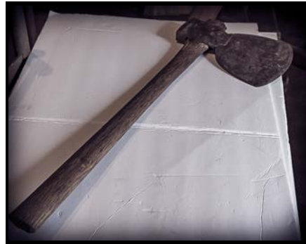
American Broad Axe (W7-19NE): Forged iron with poll, straight wood handle. Has manufacturer's stamp. Axe style used for squaring timber logs. Early 1800s.
