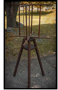
Cross-Framed Yarn Swift (P106-19S): This swift would hold a skein of yarn while it is wound into a ball or onto a spool. The holes in each of the four horizontal rods allow for adjusting the circumference. Two of the four dowels are missing and a third is broken. 1800s.
