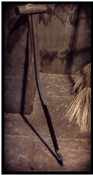
Stock Knife (P62-19NEC): Also called a Block Knife. Made of wrought iron and used in carpenter's shop to cut rough wood shapes. Would have been secured to a stump or block with a forged hook for leverage. Late 1700s.
