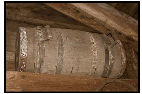
Horizontal Keg (C208-19NWR): Wooden keg for storing liquids, with metal and wood handles, metal hoops, and cork bung hole. Late 1800s.
