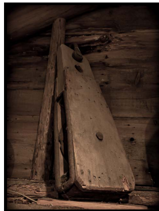
Single Sheave Pulley (M209-19WR): Large wooden pulley with iron sheave. Measurements are 30" x 10" x 4"; has an unusual trapezoid shape. 1800s.
