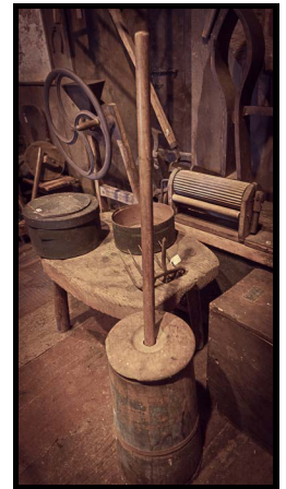
Butter Churn (P99-19NE): Tapered from bottom to top and made with staves of cedar, a butter churn might be made by a cooper.
