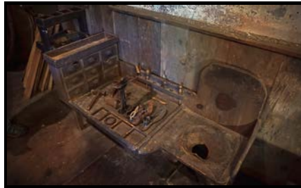
Cobbler Bench (P116-19N): Workbench and storage for making or repairing shoes and boots. Includes shoe lasts and other equipment. Late 1800s.
