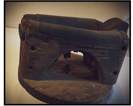
Cobbler Boot Vice (P116a-19N): Made to fit into "chair" of Cobbler's Bench, to hold boot for repair work. Late 1800s.
